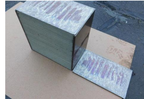
Condition analysis after hot shaker test
